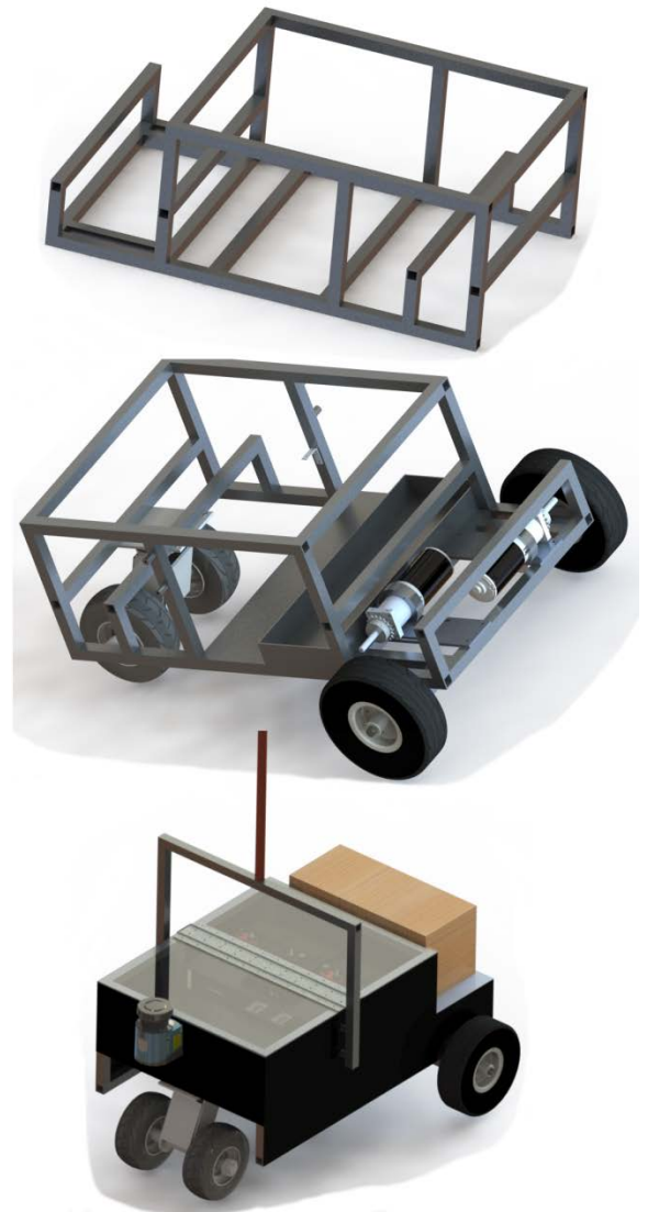
Figure 4. CAD models of the robot chassis, drive system and fully assembled.
